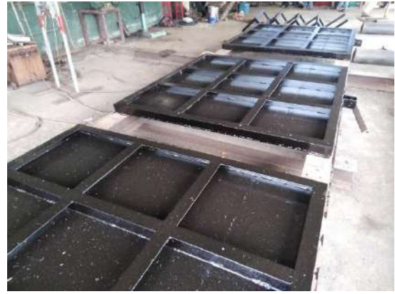
Figure 8-17: Fabrication of Radevibandiela Vertical gates
