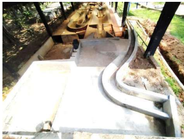
Figure 4-23: Model construction of Ellewewa uncontrolled chute spillway
