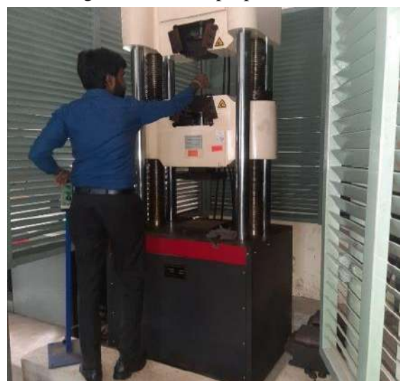
Figure 4-11: Tensile and Bending Test for Reinforcement
