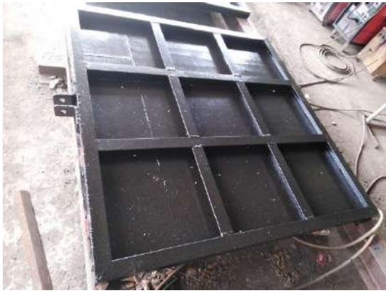
Figure 8-17: Fabrication of Radevibandiela Vertical gates
