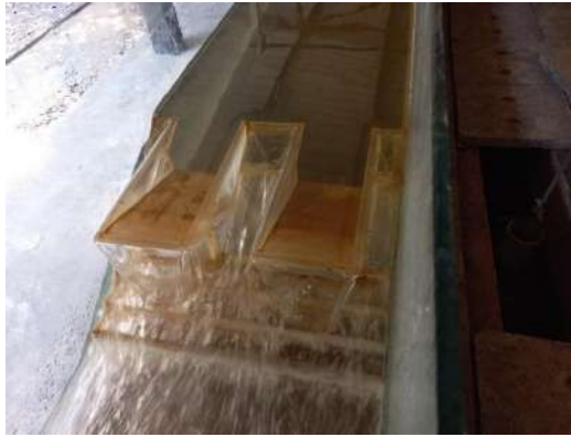
Figure 6-33: Experimental set-up - Flow over the PKW physical model with a scale of 1:20
