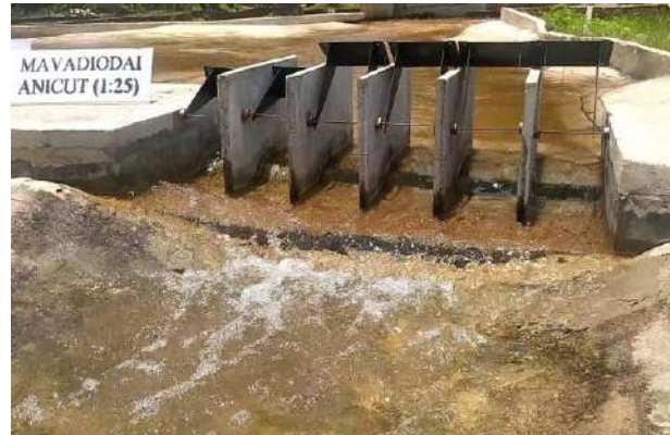
Figure 4-22: Testing condition - Mavadiodai Anicut model
